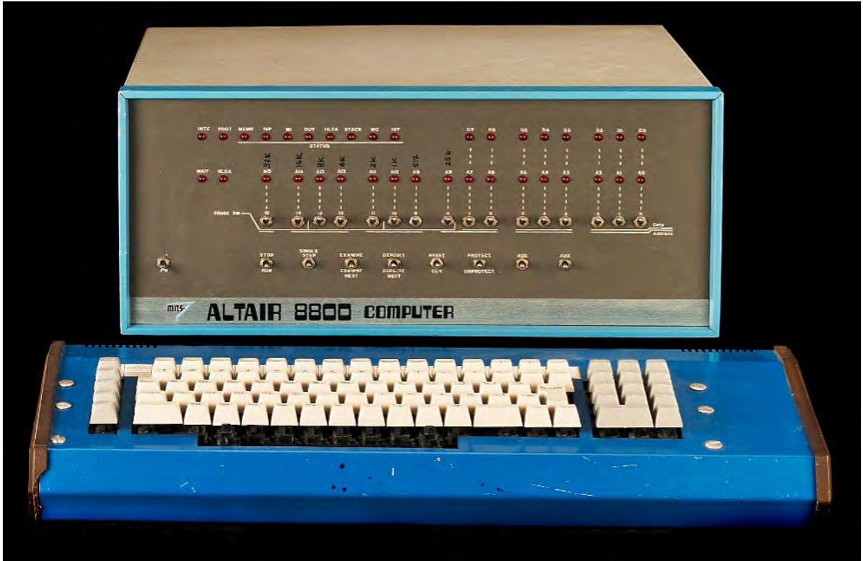
Figure 6: Early Altair 8800 model with external keyboard. Source: Smithsonian Institution, National Museum of American History.
